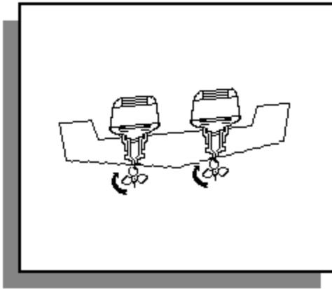
The illustration below shows how clockwise (Right Hand) propeller torque forces a boat into a right hand turn.
