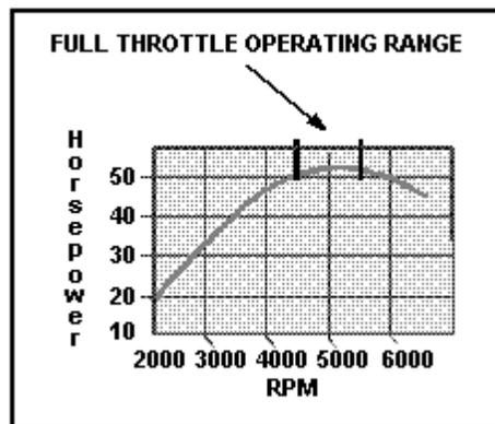
The recommended W.O.T. operating range is determined to permit operating latitudes without sacrificing engine durability or performance.
