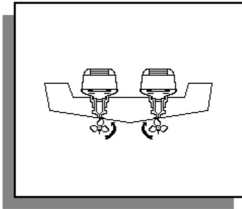
Most single engine boat setups normally operate in forward motion using clockwise rotation of the engine and gearcase. Although counterclockwise rotation setups have been used since the creation of the outboard engine, the use of **counter-rotation** has become more prevalent in the last decade. This increase is largely due to the manufacturing increase of larger **twin** engine recreational boats and performance boats.
